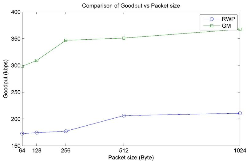
Fig. 8. Goodput vs UAV packet size
