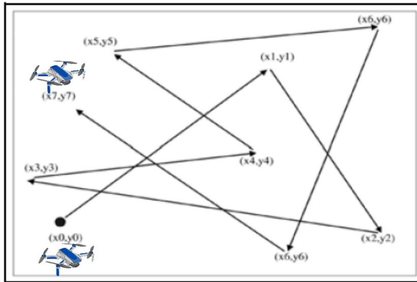
Fig. 3. Example of UAV trajectory in RWP model
