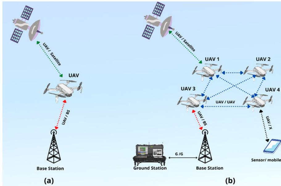
Fig. 1. (a) Single-UAV network (b) Multi-UAV network
