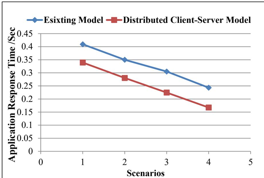
**Fig. 10.** Fixed WiMAX average application response time for the Centralized and the Client-Server models
