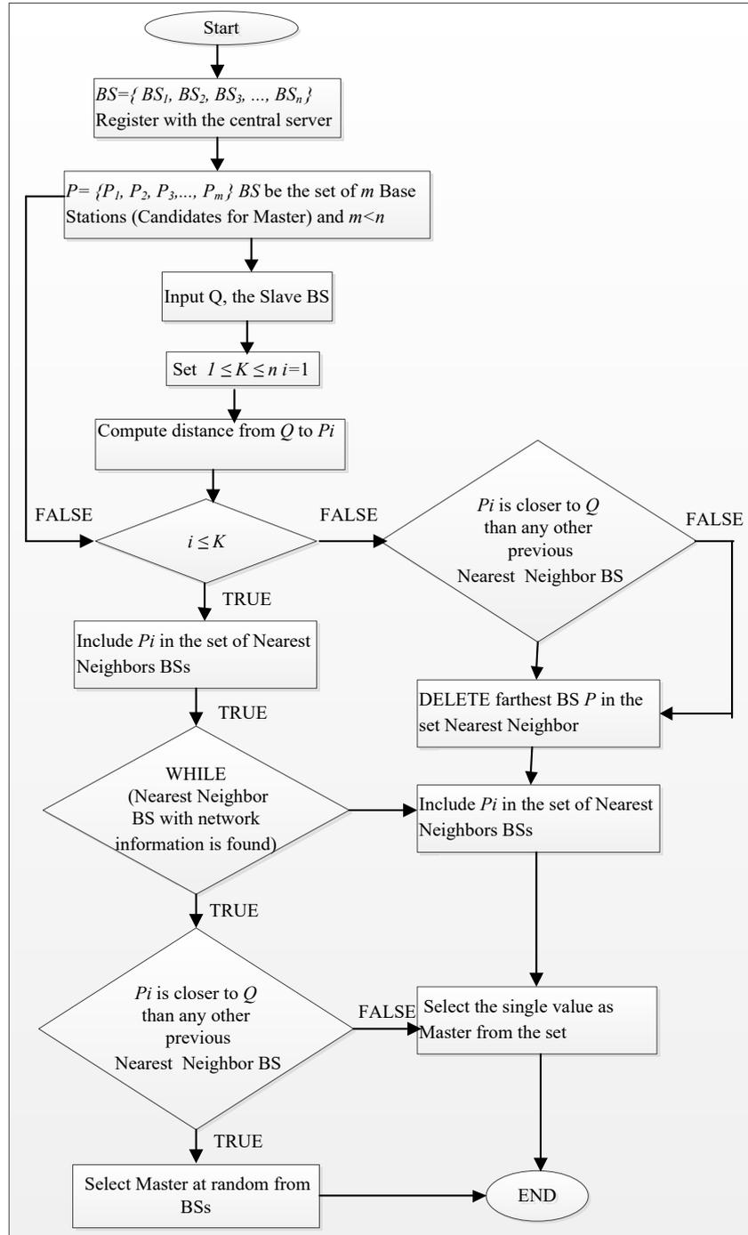
Fig. 1. Client-server BSs selection algorithm
