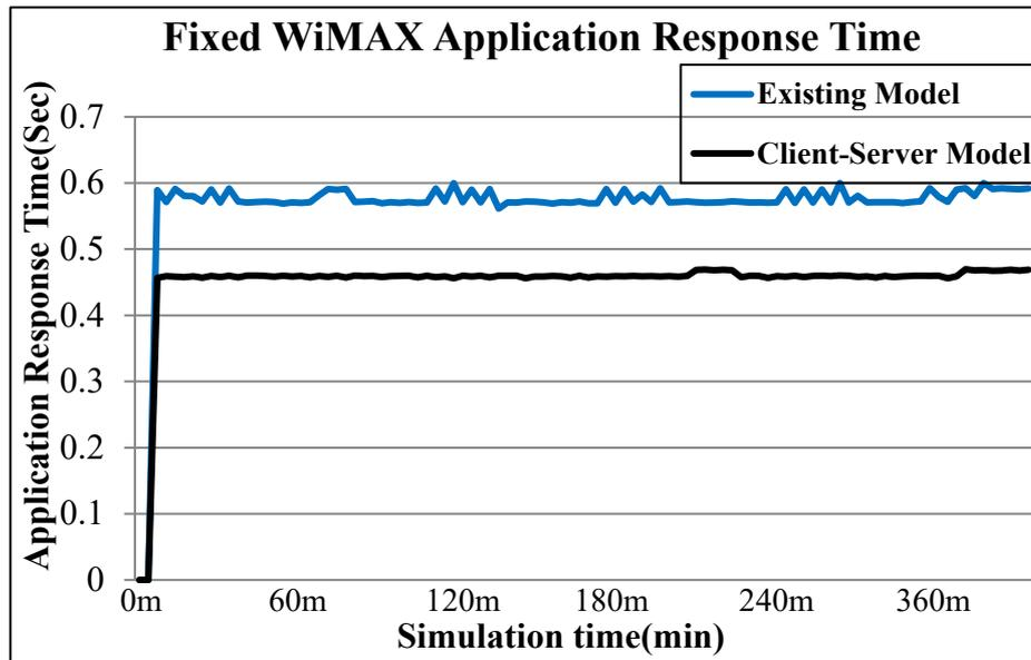
Fig. 8. Scenario 3 simulation results for the application response time comparison
