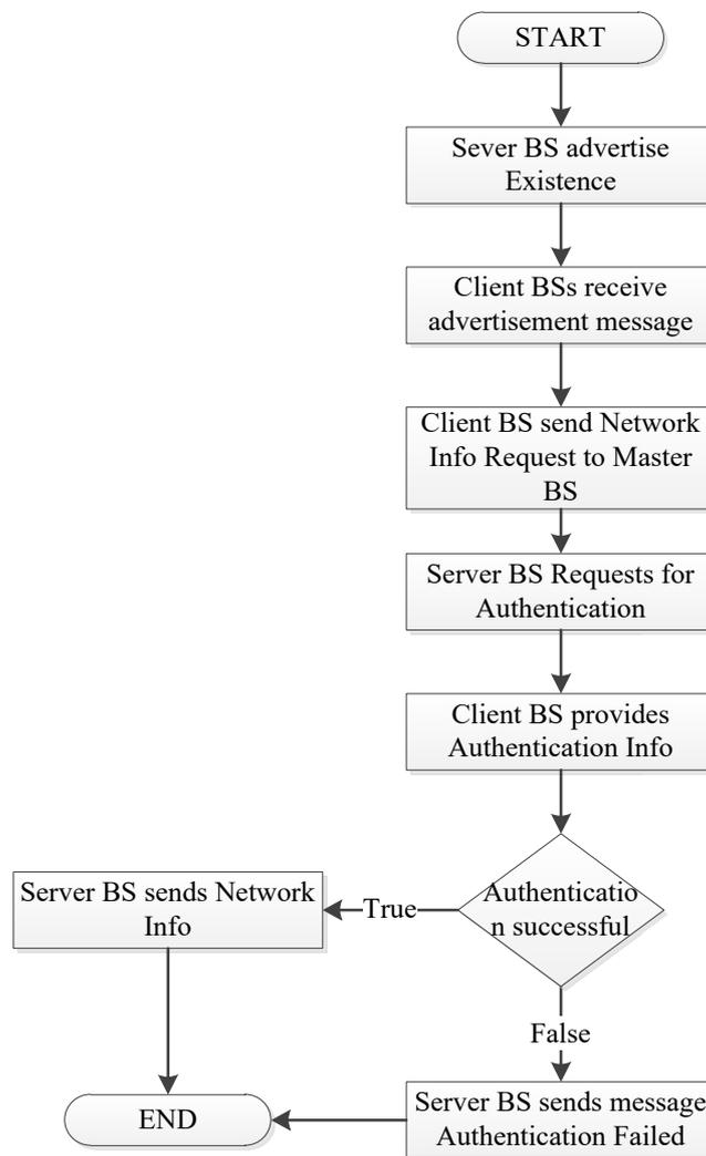
Fig. 2. Client-server BSs communication algorithm
