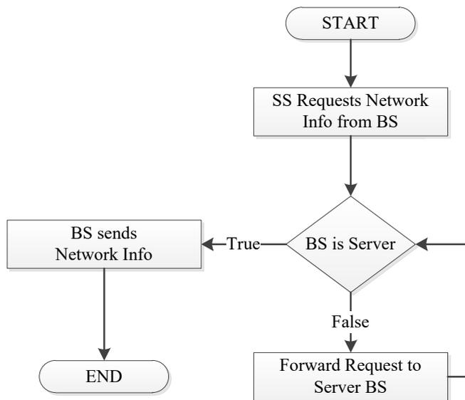
Fig. 3. Base station and subscribers stations communications algorithm
