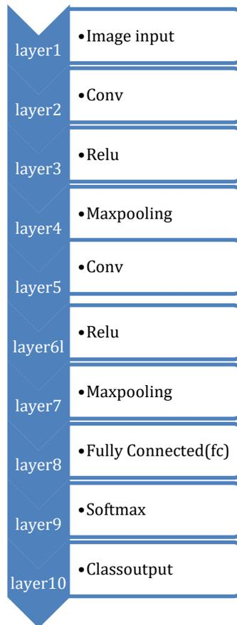
Fig.7.CNN-layers diagram for iris recognition [5]
