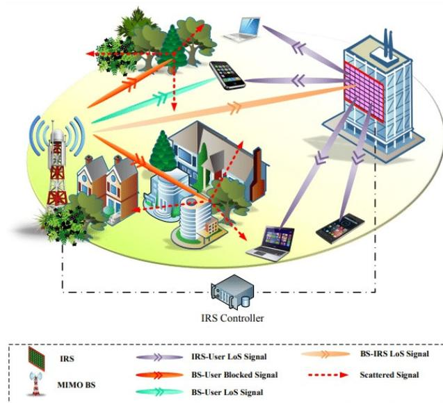
**Fig. 2.** Metasurface real time interface for signals between transmitter and receiver using the IRS controller [17]
