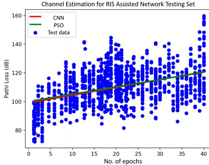
Fig. 6. Testing set stage for channel estimation of RIS-aided network
