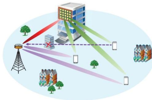
**Fig. 1.** An example on Reconfigurable Intelligent Surfaces (RIS) wireless communication system [10]
