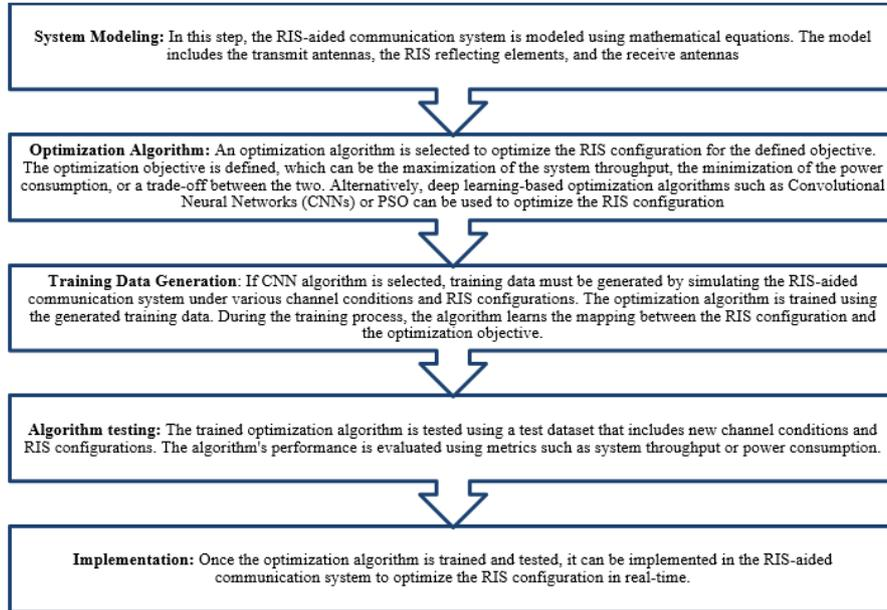
**Fig. 3.** This represents the steps accumulated for the RIS-aided communication between the transmitter and receiver
