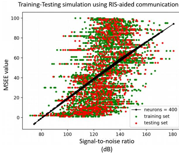
**Fig. 8.** This simulation contains the MSE value vs the SNR required for the channel estimation performance
