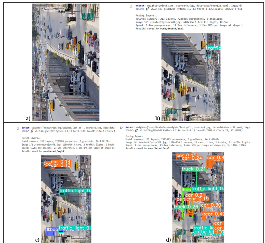
Fig. 10. The detections of an object rotated 90° (a) rotated input image (b) by the original model (c) by the proposed model without change image degree model (d) by the proposed model with change image degree
