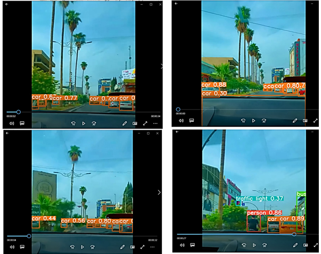
Fig. 11 Results of object detection in the video using YOLOv5
