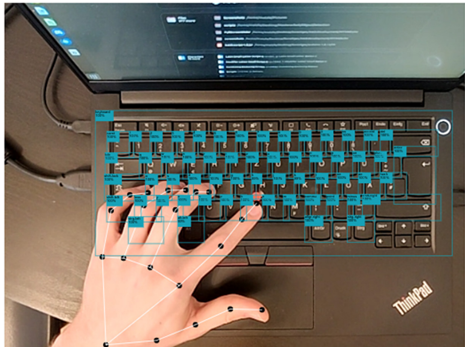
Fig. 6. Position comparison of the key detection bounding boxes and finger positions of the hand pose estimation
