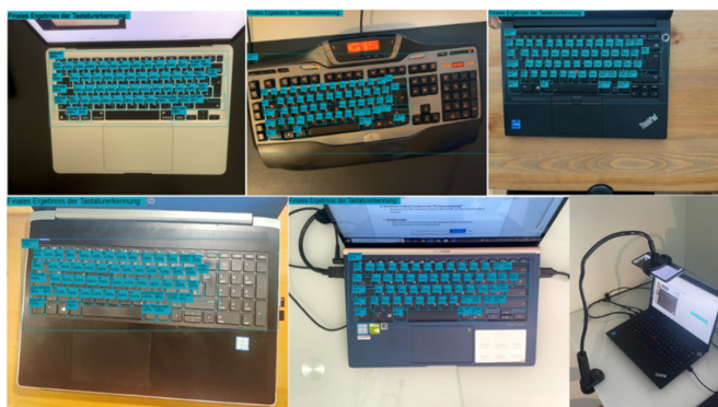
Fig. 4. Final result of the implemented key detection model based on the EfficientDet architecture for different test persons
