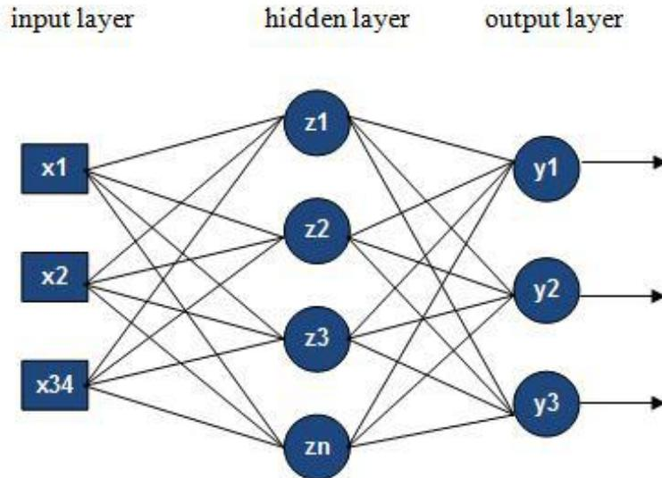
Fig. 2. Backpropagation neural network architecture
