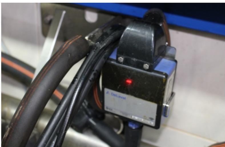
**Fig. 3.** Milk Meter Appliance.
