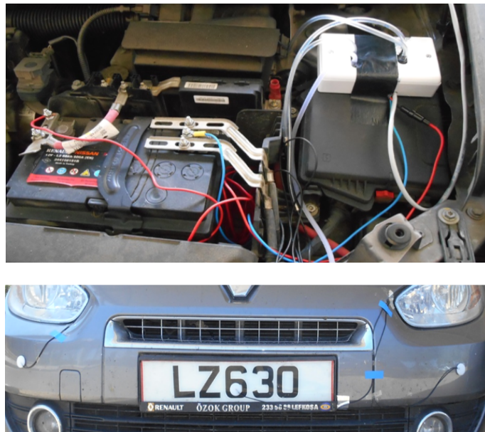
Fig. 3. Images of the pressure sensors box in the engine compartment and the pressure ports in the front of the car
