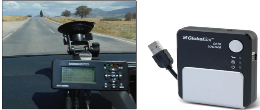
Fig. 4. OBD II Dash Dyno logger and GlobalSat GPS logger
