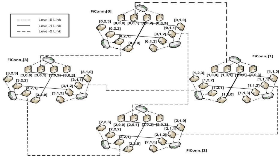
Fig. 5. A FiConn Interconnection Structure with  $n = 4$  [28]
