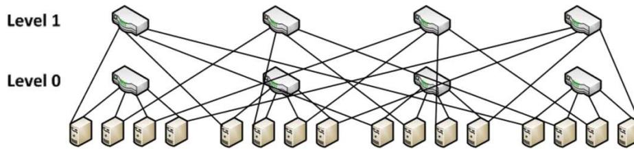
Fig. 4. A BCube Interconnection Structure with  $n = 4$  [31]
