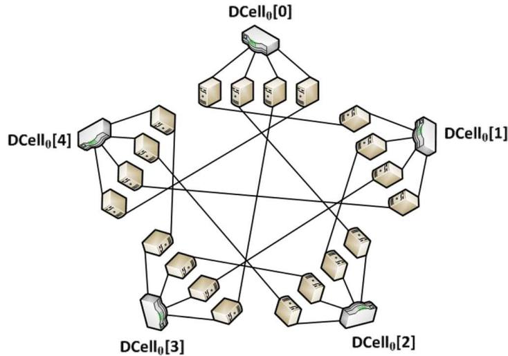
Fig. 3. A DCell Interconnection Structure with  $n = 4$  [29]
