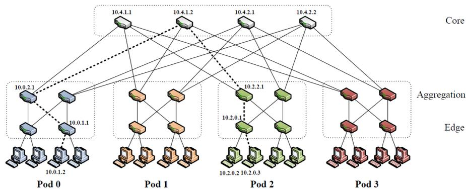
Fig. 2. A Fat-Tree interconnection Structure, with  $n = 4$  [22]
