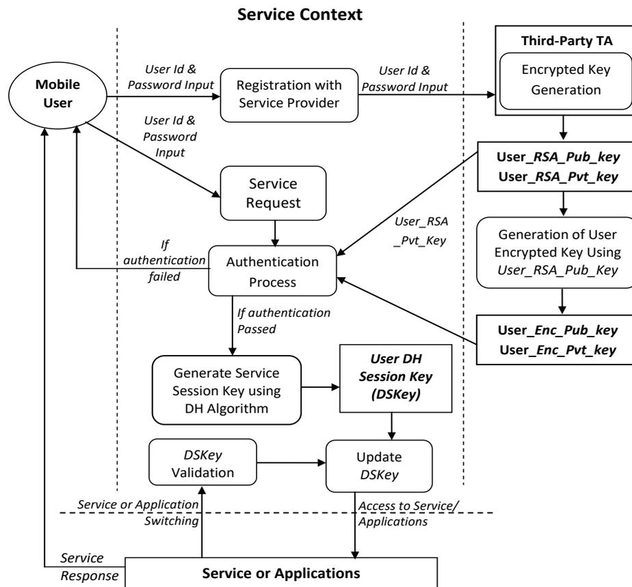
Fig. 1. Proposed Authentication Architecture
