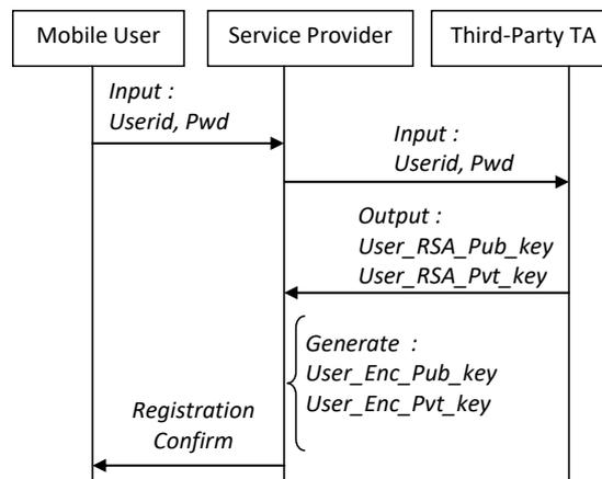
Fig. 2. Registration Process and Key Generation
