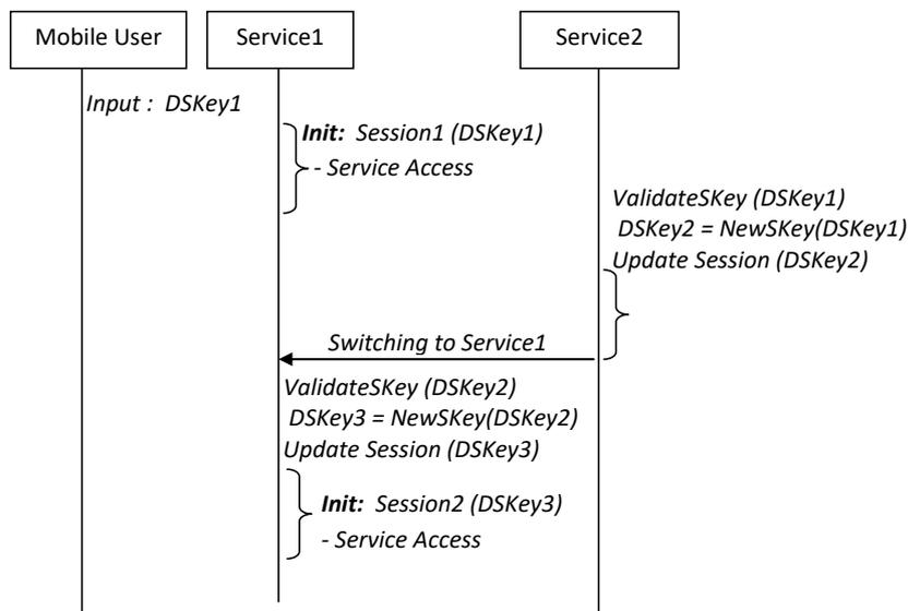
Fig. 3. An Illustration of DSKey Exchange Mechanism
