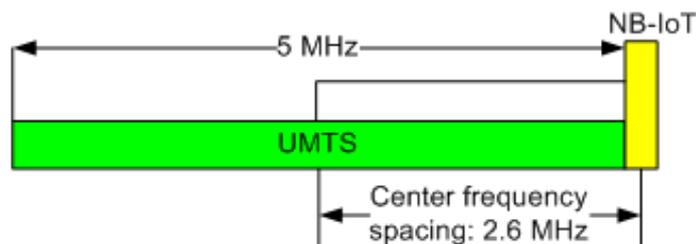
Fig. 5. NB-IoT deployment on UMTS idle spectrum resources
