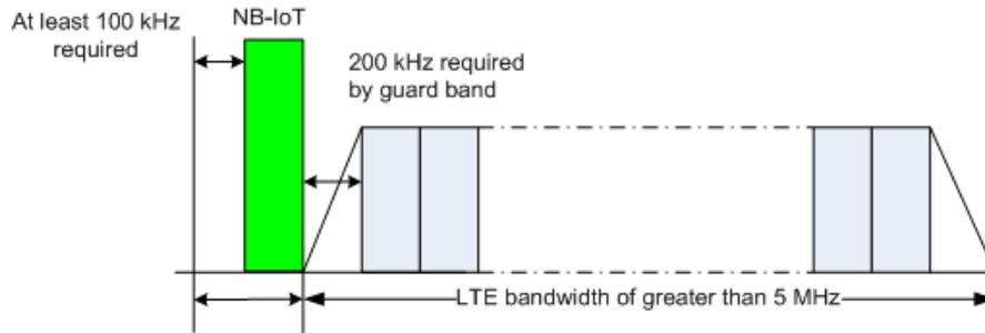
Fig. 6. NB-IoT deployment on LTE idle spectrum resources
