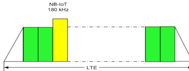
**Fig. 9.** LTE In-band deployment
