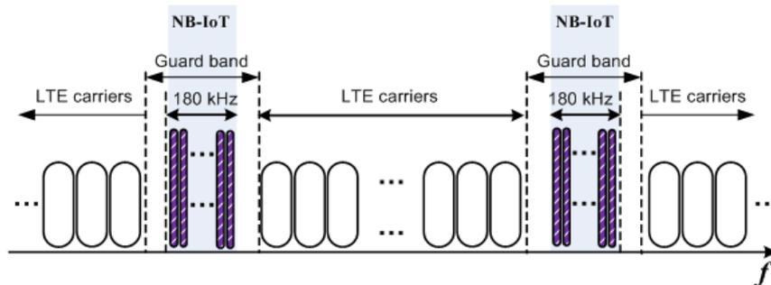
Fig. 7. LTE guard band deployment
