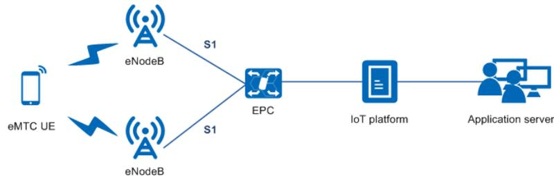
**Fig. 10.** eMTC network architecture
