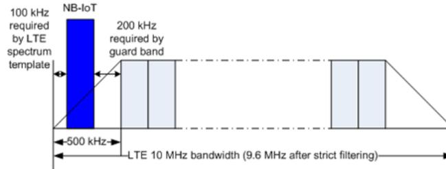
**Fig. 8.** LTE guard band deployment
