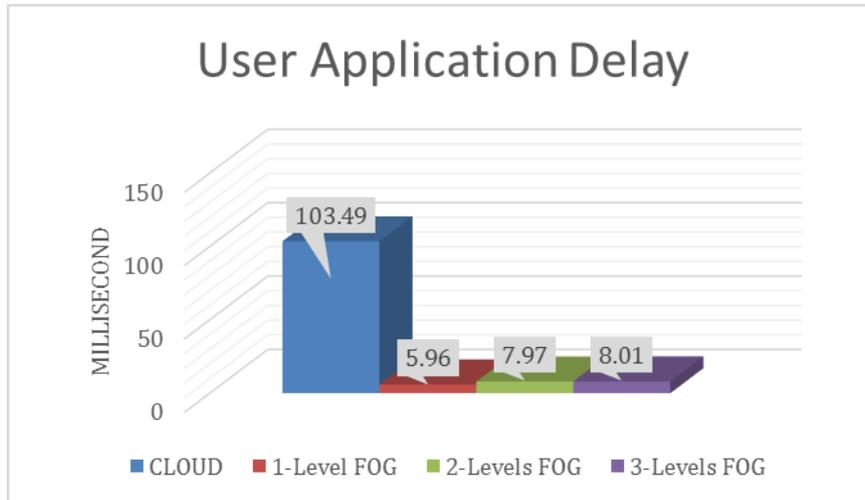
**Fig. 6.** Application Delay of Multiple Architecture of Proposed Parking System Compared to Cloud-Computing Paradigm
