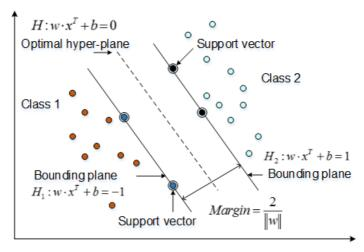
Fig. 1. Optimal separating hyper-plane for data classification
