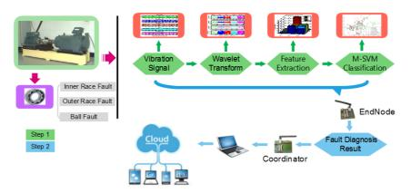
Fig. 2. The overall architecture of the proposed system
