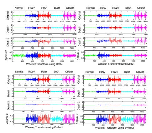
Fig. 6. The 2-level DWT decomposition of the vibration signals under five bearing working conditions using four different mother wavelets
