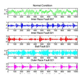
Fig. 3. The original vibration signal of the bearing with different conditions
