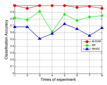
Fig. 10. Comparison of the classification accuracy of the proposed approach with neural network and minimum distance methods
