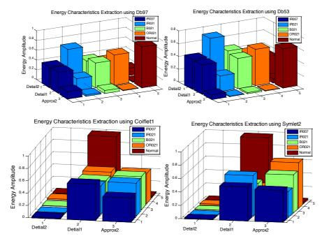
Fig. 7. The normalized energy of wavelet coefficients for vibration signals under five bearing working conditions using four different mother wavelets
