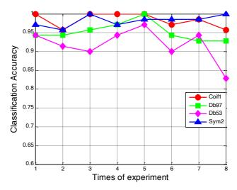
Fig. 9. Comparison of fault diagnosis classification accuracy using different wavelet
