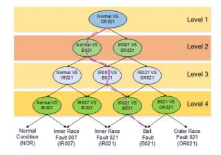
Fig. 5. The DAG for selecting the correct machine working condition out of five classes
