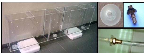
Figure 3. Acrylic tank and pressure tap accessories.
