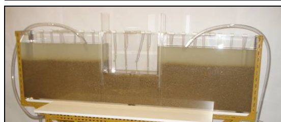
Figure 4. Seepage into a double-walled cofferdam.
