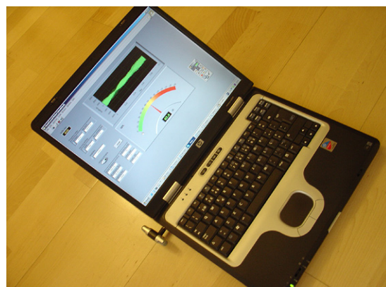
Figure 6. Computer with microphone running the SPL meter emulator software
