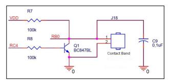
Figure 5. Schematic for the contact bands.
