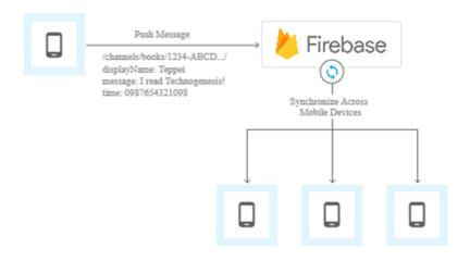
Fig. 4. Push messaging device to device [1]
