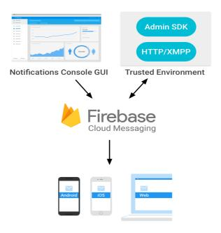
Fig. 1. Firebase cloud messaging Architecture [1]
