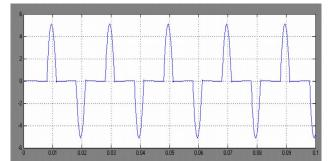
Fig 3a TCR Current Waveform with Alpha = 144 Degree
