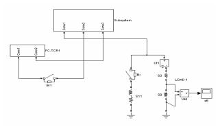
Fig 5 (b) Three bus system with FC-TCR
