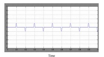
Fig 2a TCR Current Waveform with Alpha = 162 Degree
