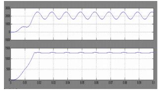
Fig 3b Real & Reactive Power with Alpha = 144 Degree
