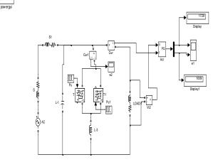
Fig.1b.Circuit model of FC- TCR
