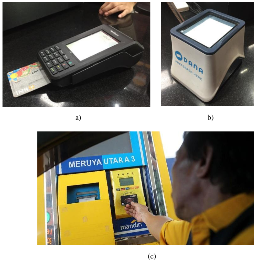
Fig. 1. Commercial device of portable electronic transaction: (a) contactless; (b) contact smart card; (c) toll payment device that uses a contactless smartcard
