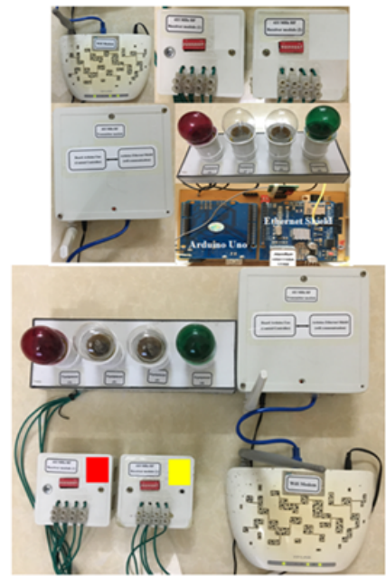
Fig. 2. The experimental model using two channels including RF315 module and wifi Shield module
