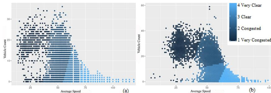
**Fig. 4.** Clustering result of (a) road 158324 traffic condition, (b) road 193294 traffic condition
