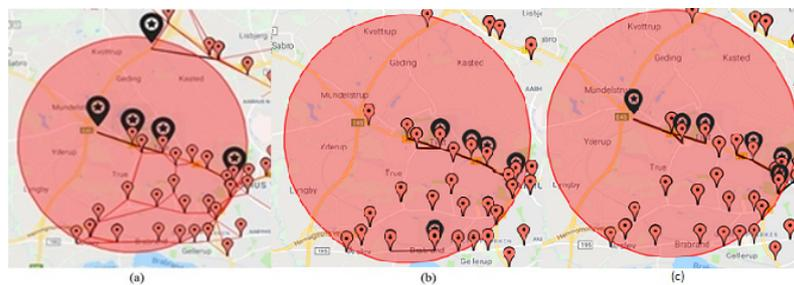
**Fig. 7.** Map plotting of results for road 158324 with its neighbouring roads (a) using correlation method (b) using k-means and (c) using k-NN.
