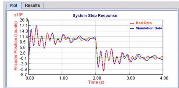
Figure 11. Comparison of real and simulation results (rigid plant)
