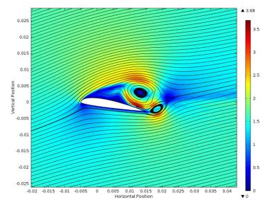
Fig. 4. Module 3 (IBL: Biomimetic Flight, Student A, Velocity Field in Plunge Cycle)
