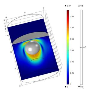
Fig. 3. Module 2 (Transitional): Oil Bubble in Water
