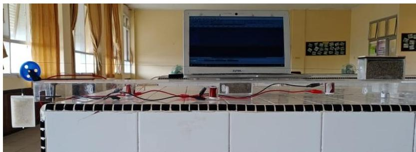
**Fig. 1.** The experimental setup consists of a trajectory table made of rough acrylic
