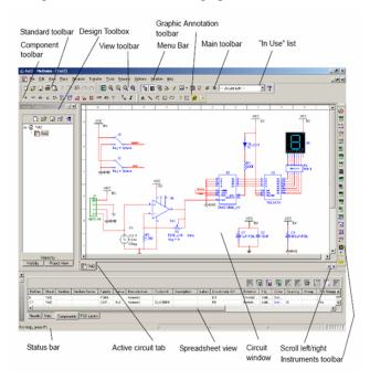
Figure 1. Display of Multisim Environment
