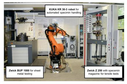
Fig. 2. Tele-operative testing cell at the IUL in the current expansion stage with two testing machines and one robot for automated test specimen handling
