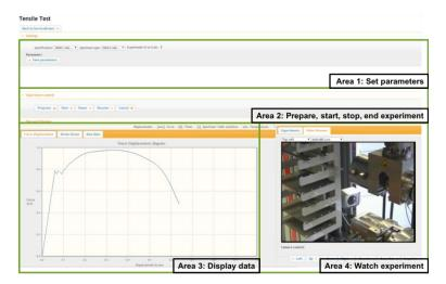
Fig. 3. Graphical web interface for operating the testing cell
