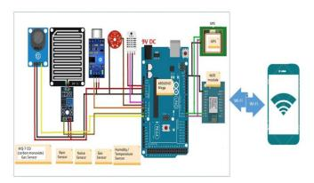
Fig. 4. Diagram of the Complete System.
