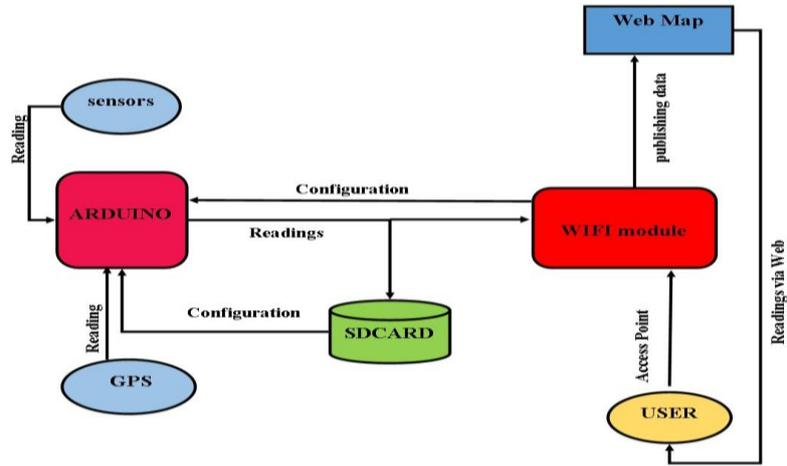
Fig. 3. Station Architecture.
