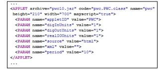
Figure 3. Integration of the PWC applet into an HTML page
