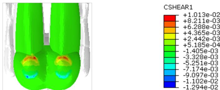
Fig. 8. Shear stresses at the interface buttock-thigh tissue
