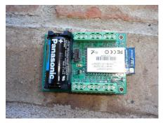
Figure 2. Tag4M tag powered from a 3V Lithium battery
