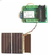
Figure 4. Tag4M tag with solar cell connected directly to tag power terminals
