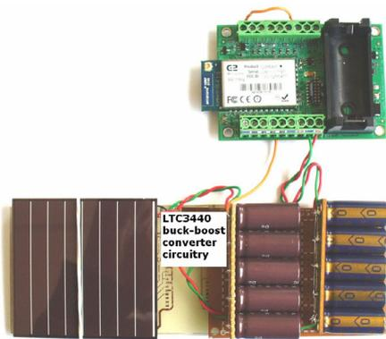
Figure 7. Tag4M tag with solar cell connected to capacitor array via a buck-boost converter circuitry
