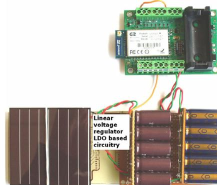
Figure 6. Tag4M tag with solar cell connected to capacitor array via a linear voltage regulator
