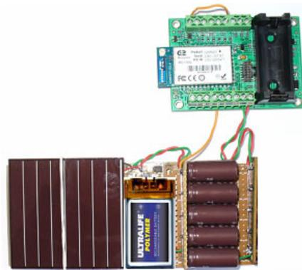
Figure 8. Tag4M tag with solar cell connected to capacitor array via a buck-boost converter circuitry, Li-Ion Accumulator and charger
