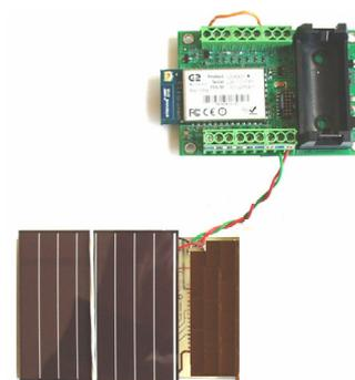
Figure 4. Tag4M tag with solar cell connected directly to tag power terminals
