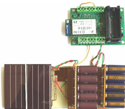
Figure 5. Tag4M tag with solar cell connected to capacitor array
