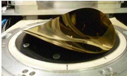
**Fig. 1.** Warpage observed on low thickness wafer
