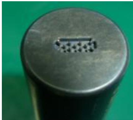
**Fig. 10.**Ejectorless cavity
