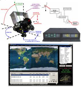
Figure 4. SRT positioning subsystem: Engines (upper left) and digital controller (upper right) [26] and Orbitron tracking software (down) [38].
