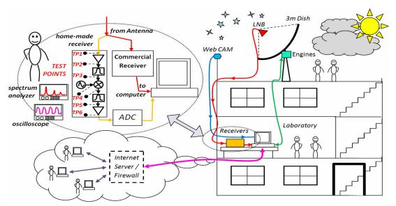
Figure 2. Scheme of the Radio Astronomy & Microwave and Antenna Engineering Laboratory
