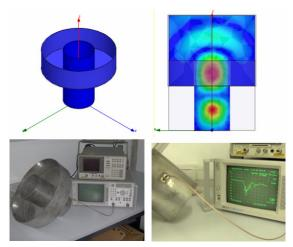
Figure 8. Development of the SRT horn feeding the parabolic reflector
