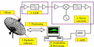
Figure 3. Scheme of the SRT RF system and subsystems
