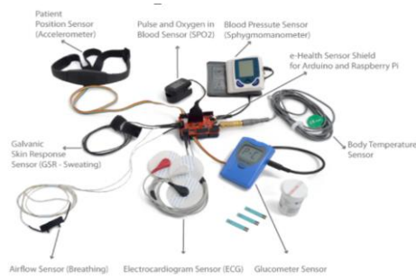
Fig. 11.: Sensors connected Raspberry Pi
