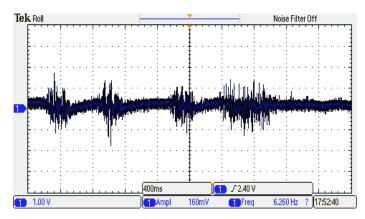
Fig. 16. The Output of Summing Amplifier Circuits
