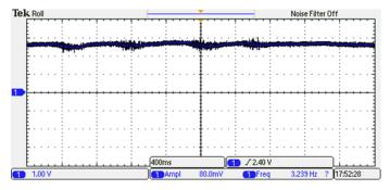
Fig. 15. The Output of Myoware Muscle Sensor
