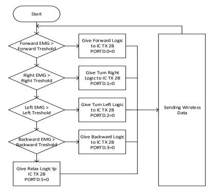
Fig. 3. Diagram Comparator System Flow
