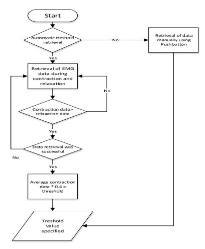
Fig. 4. Flow Chart Determination of Threshold Value
