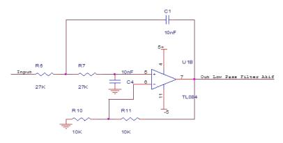
Fig. 7. Low Pass Filter Circuit
