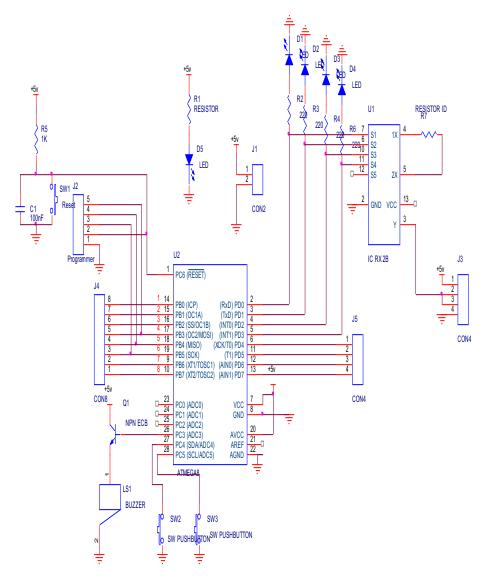
Fig. 13. Minimum System Receiver
