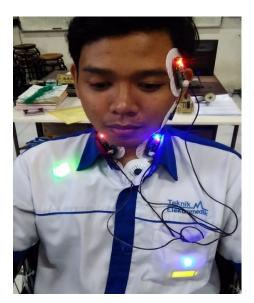
Fig. 22. Position of the EMG Signal Tapping Electrodes
