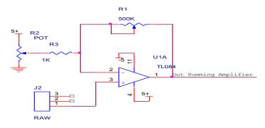
Fig. 6. Summing Amplifier Circuits
