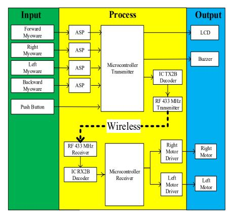
Fig. 2. Block Diagram of Electronic Systems
