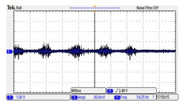
Fig. 18. The Output of High Pass Filter Circuit
