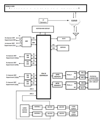
Fig. 1. Architecture of M-learning based remote laboratory setup
