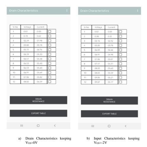
Fig. 5. JFET CS drain characteristics readings
