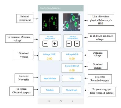
Fig. 4. Android mobile application screen for JFET CS configuration
