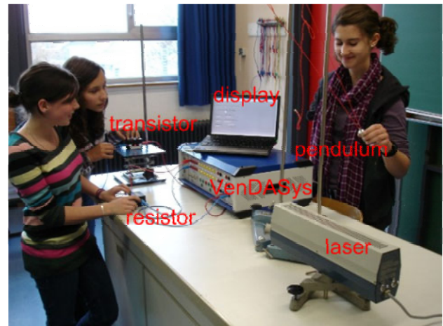
Figure 16. Experimental set-up for measuring the oscillation period of a pendulum with a laser beam and phototransistor.
