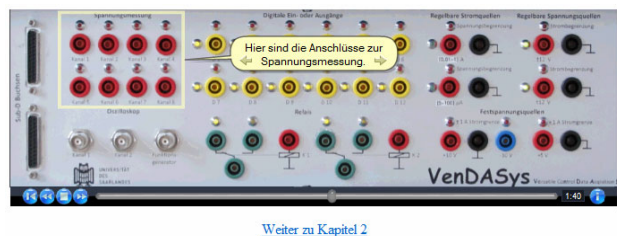
Figure 19. Screenshot of a flash video from the VenDASys self-study course; here, the function of the different front panel connectors is explained, marked are the connectors for voltage measurements.
