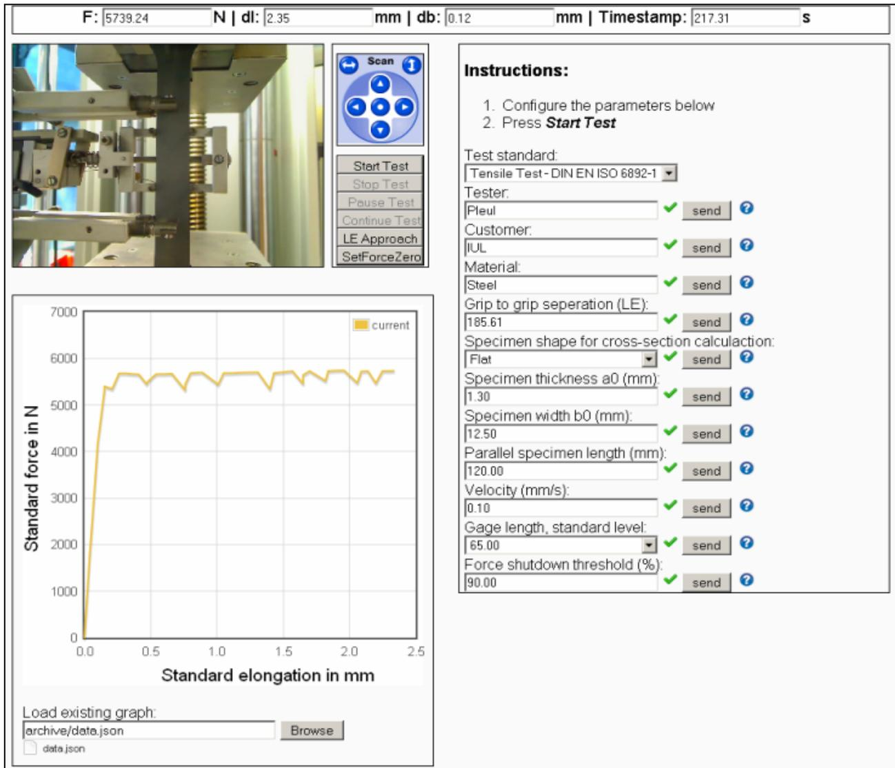
Figure 2. In-house developed interface of tele-operated tensile test: real-time values (top bar); video stream with buttons to control and interact with the experiment (upper left); set-up panel for test configuration (right); real-time diagram including access to the test archive (left)
