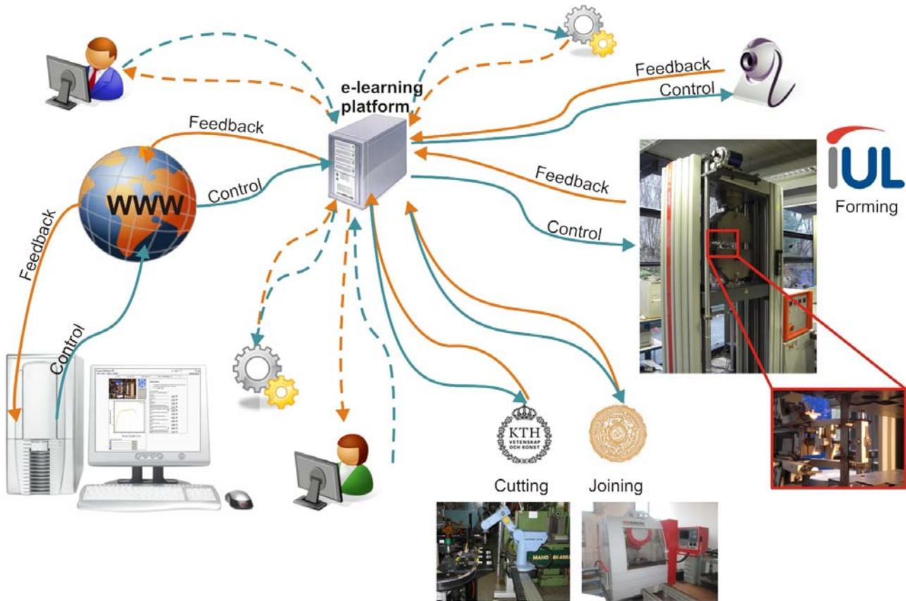
Figure 1. Principle framework of the overall PeTEX system. Tele-operated experiments like tensile test, cutting, and welding are connected with the e-learning platform by Internet. Learners can access the learning environment with the integrated experiments accessible via the e-learning platform on their computer screens.
