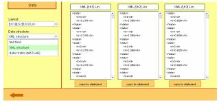
Figure 8. Data export from measurement. User can choose between three types of data structure (plain text, XML, and MATLAB matrix)
