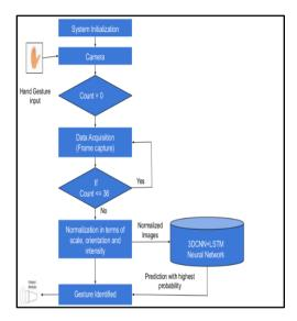
Fig. 5. Block diagram for dynamic gesture recognition
