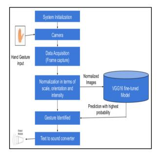
Fig. 4. Block diagram for static gesture recognition
