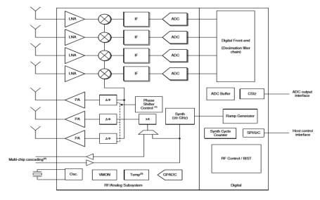
Fig. 5. AWR2243 functional block diagram
