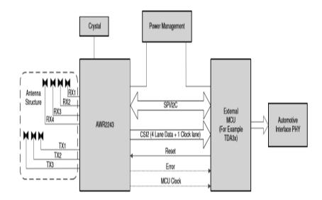
Fig. 4. Interfacing External host to AWR2243
