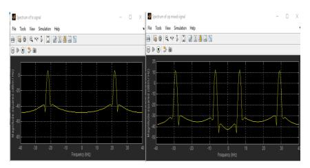
Fig. 2. Transmitted signal(left) Output Mixed signal (Right)
