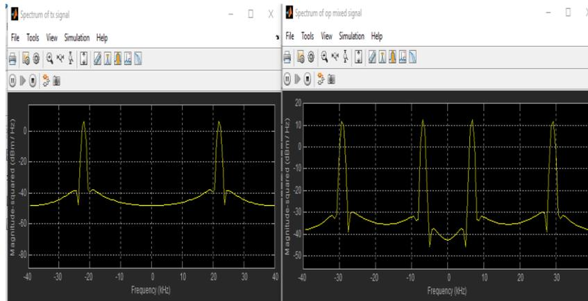
**Fig. 2.** Transmitted signal(left) Output Mixed signal (Right)
