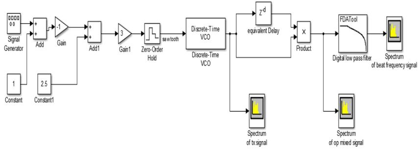
**Fig. 1.** Illustration of FMCW concept
