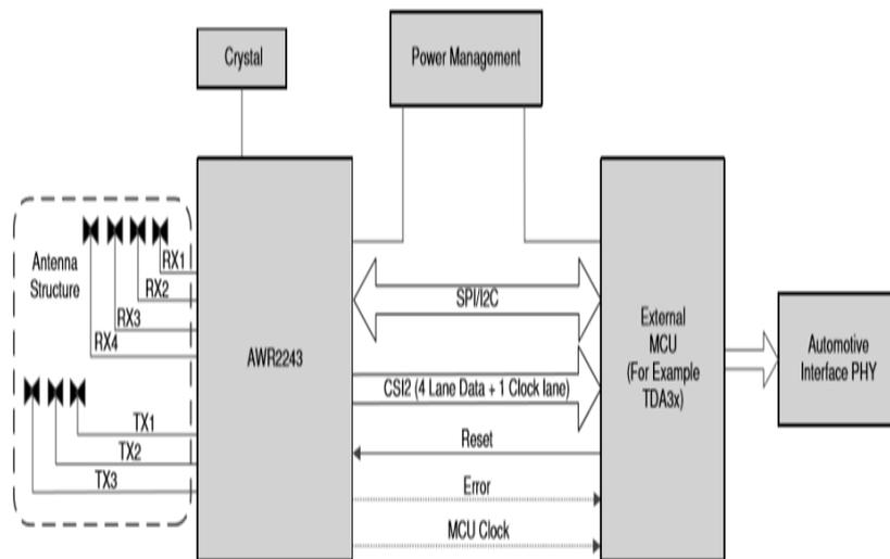
**Fig. 4.** Interfacing External host to AWR2243
