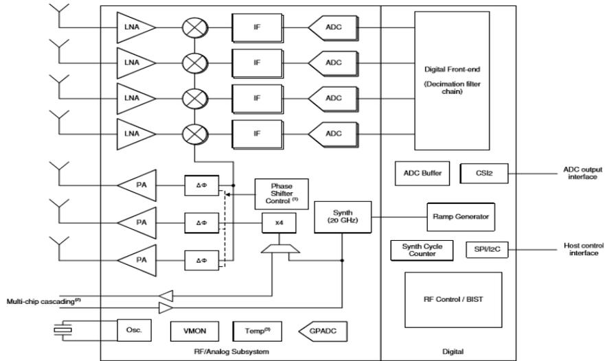
Fig. 5. AWR2243 functional block diagram
