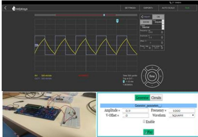
**Fig. 11.** Charging and discharging of a capacitor using the remote IoT system
