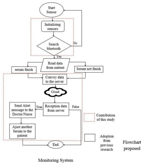
Fig. 2. Flowchart of the proposed Smart Monitoring System
