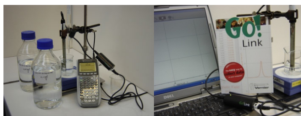
Figure 1. TI-84Plus™ + peripherals EasyLink™(left) + Go!Link™ (right)
