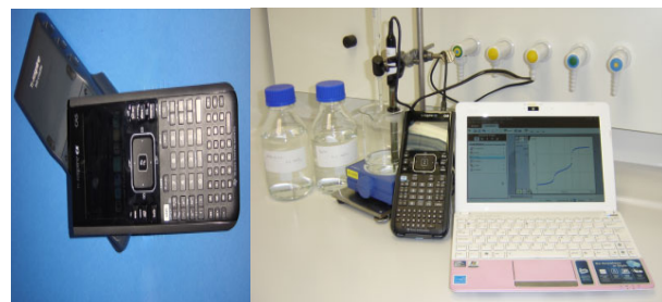
Figure 2. TI-Nspire cx CAS™+ lab cradle™ (left) in combination with computer (right)
