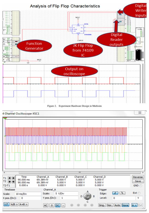
Figure 3. Frequency Division Simulation Results
