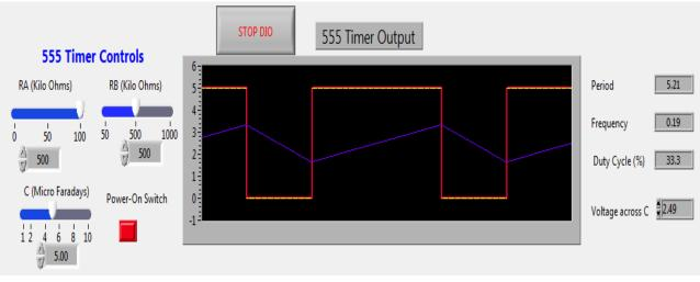
Figure 8. 555 Astable Circuit Analysis
