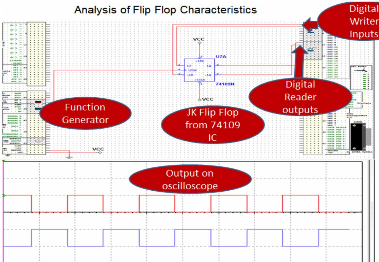
Figure 2. Experiment Hardware Design in Multisim
