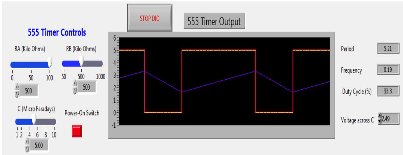
Figure 8. 555 Astable Circuit Analysis
