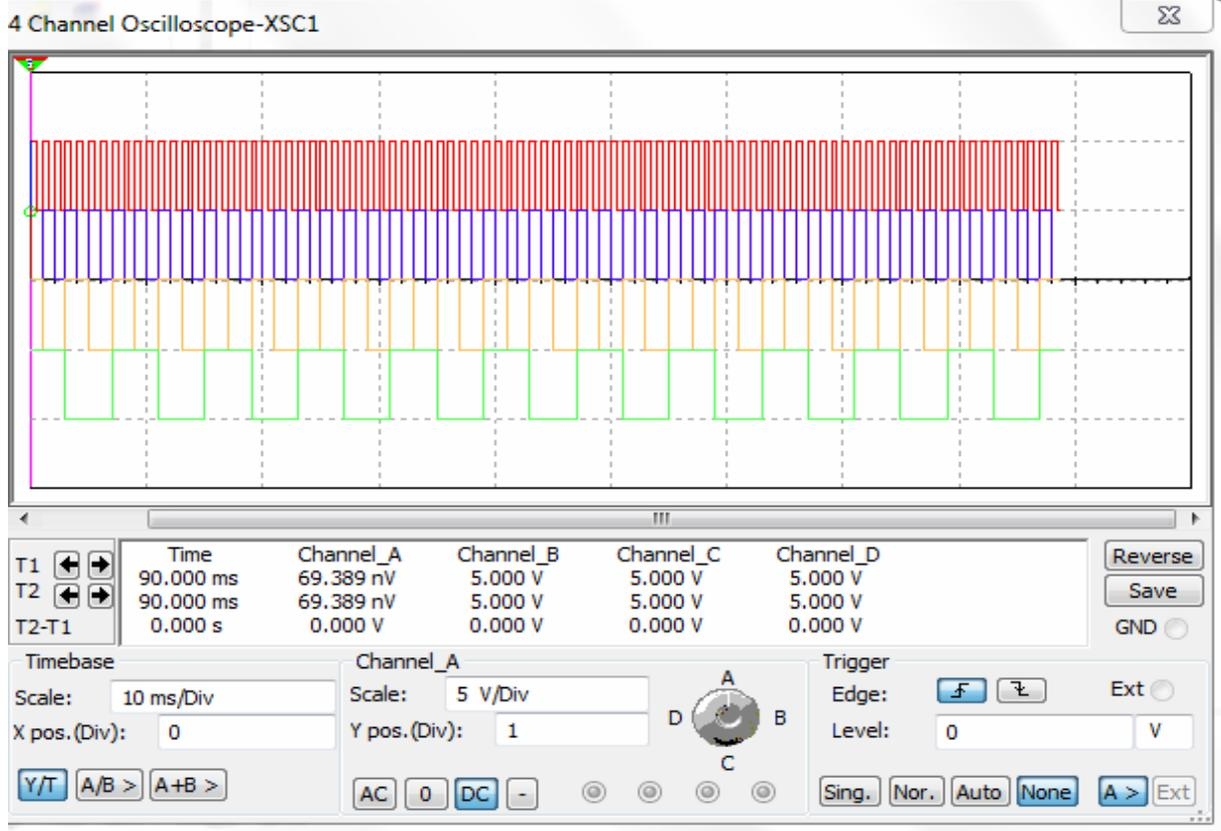
Figure 3. Frequency Division Simulation Results
