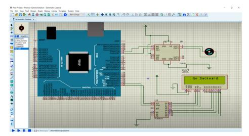
Fig. 5. The Dc motor control on the Proteus simulator
