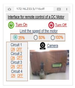
Fig. 4. The developed interface for the remote control of the DC motor
