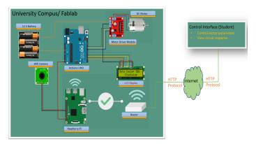
Fig. 2. The adapted architecture for the remote control of a DC motor
